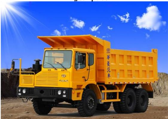
Cabin:European style,interior upgrade entirely,cabin air spring suspension system,the safety air chamber for drivers. The steering wheel adjustable for different people. The big power A/C system can fulfill the rough working conditions. The artomatic and hydraulic tilting system is for easy maintenance.
